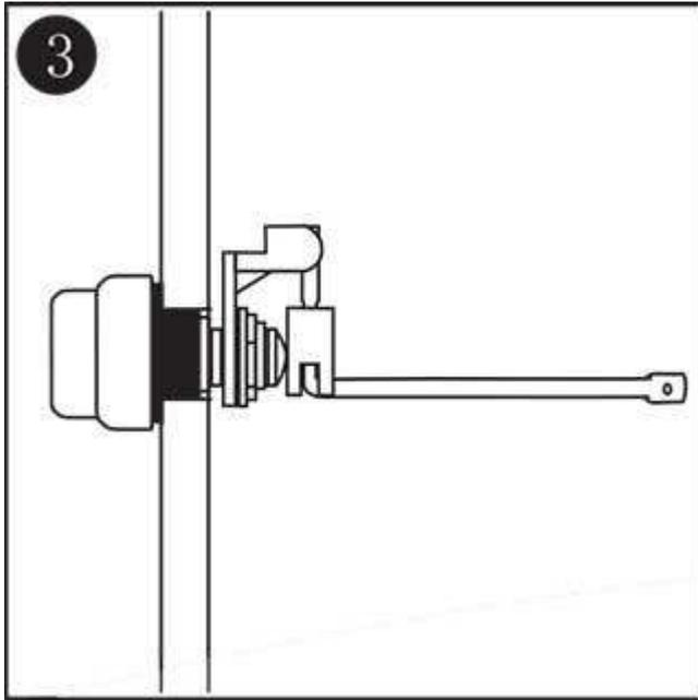
Attach the stand rod on and screw the nut tight.
