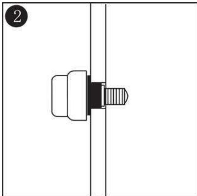
Put the push button into the tank lever hole.
