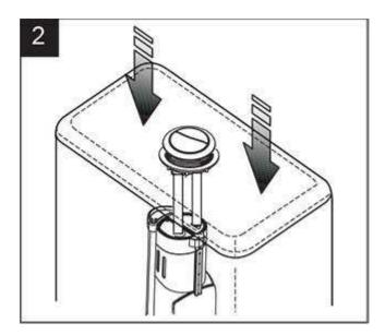
2.Adjust the direction of the push button. Be sure the full flush button towards the full flush touch piece.
