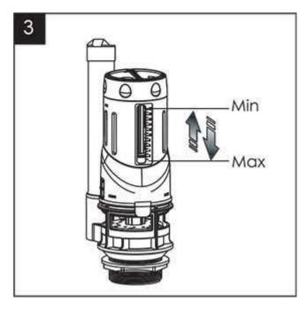
3. Adjustment of partial flush level: The partial flush float is higher, the partial flush water is less.
