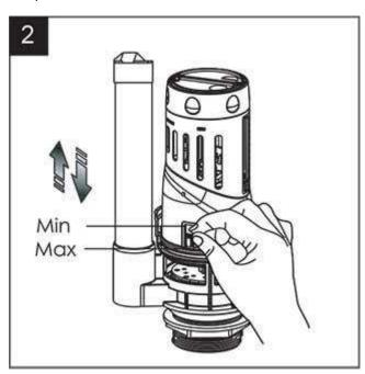
2. Adjustment of whole flush level: When the red card is on highest position, the whole flush water is at the least.
