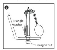
1. Spin the hexagon nut open, take off the plastic pad and Insert the fill valve into the water-in hole of the tank, make sure the triangle washer is at the position as the drawing show.
