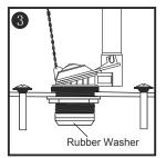
Put the tank on the toilet bowl, make sure the tank rubber washer exactly center over the flush open. Use the tank bolts to install the tank and the toilet bowl.
