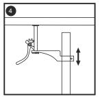
Move the connector up and down and rotate the connector ,make sure the movable rod center over the push button hole and the height is suitable.
