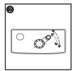
Adjust the angle of the flush valve, make sure the flapper is easy to open, and the chain is not blocked.
