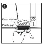
Take the nut&plastic flush washer, put the flush valve center over the flush open at the bottom tank. Make sure the triangle gasket is between the tank and the flush valve.
