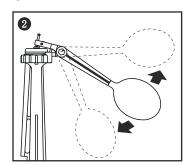
2.Adjust water level by loosening thumbscrew located at the base of the float rod. Position adjustable float rod to desired height, then tighten thumbscrew. Turn on water and check for leaks.
