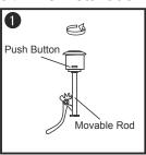
Screw the push button away from the movable rod counter clockwise.
