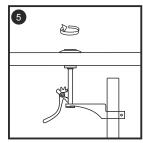
Put the push button into the upper tank hole,screw the movable rod. When the gap between the push button and tank is too big,adjust again according to the drawing.
