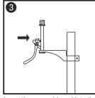
Insert the moveable rod into the connector rod.
